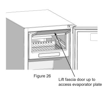
Refer to your cleaning solution instructions to determine the proper amount of cleaning solution to add based on 2 quarts (1.9 liters) of water. Lift fascia door up to access evaporator plate. (See Figure 29). Pour the cleaning solution slowly on the evaporator plate so it flows down into the fresh water reservoir. (See Figure 30).
