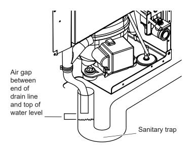
Figure 13: Example of an open drain.
